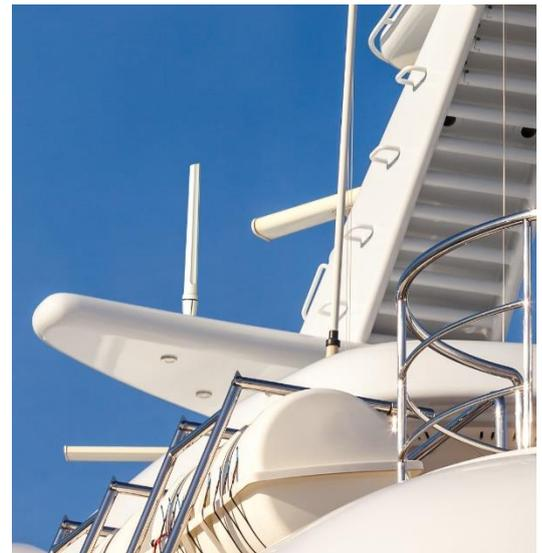
The OMNI-402 marine antenna offers a standard 1"-14TPI marine adaptor (BRKT-40 in the box) and can optionally provide a standard 1¼"-11TPI marine adapter (BRKT-41) where these larger mounting points are already installed on the yacht or boat. A series of optional 316 grade stainless steel marine mounts are available, namely the BRKT-37, BRKT-38 & BRKT-39.
